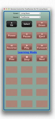
Once the code has been entered properly, click the "OK" button. The programming window will close. The button on the remote control panel is now updated. Click the next button to continue programming. Once programming is complete, press the escape key to exit learning mode.
