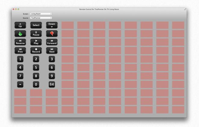
Changing the source in the pull down on this widow performs the change in the video matrix for that screen as well. So it is conceivable that this window could be used full screen and all operations controlled for it. As with the smaller remote panel, each screen can have its own unique buttons for each source allowing for a very large number of devices to be controlled.
