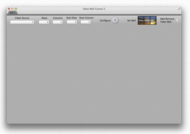
Upon creating a new video wall control, the video wall control window is displayed. The initial display looks as shown to the left. Screens will need to be assigned to the wall, so click on the "configure" button. The video wall configuration window will open. In the upper right set the number of rows and columns. The number of screens will adjust. Then select which screen is assigned to each spot in the video wall.
